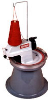
The Hague D280 Linking Machine is available in 3 different gauges, standard 7pt, fine 10pt, and fine 12pt.
